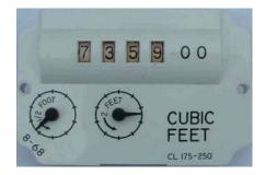
This meter has measured 735900 cubic feet, or 7359 units (CCF) of natural gas. To obtain the amount of gas you have used since your last bill, subtract the amount on the last bill (for example 7349) from the amount read from the meter. In this example, you would have used 10 units of natural gas since your meter was read the last time.
